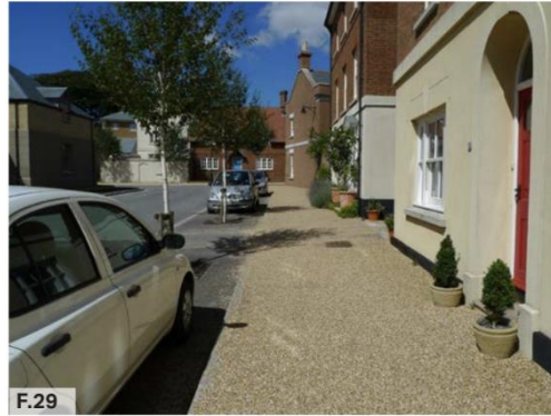
Figure 29: Example of on-street parking with parking bays and street trees to mitigate the impact of the cars on the streetscape, Poundbury.
